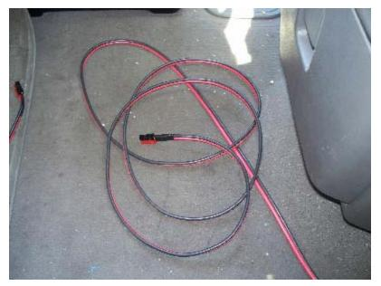
Route the power cable into the area where you plan to mount or lay your radios, bearing in mind you might have a cooler, or other containers with liquids, in the same area during the trip.
