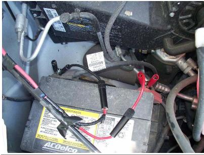
When done, don't forget to actually connect the battery under the hood using the cable clamps, then secure the cable from vibration using electrical tape or nylon wire-ties.
